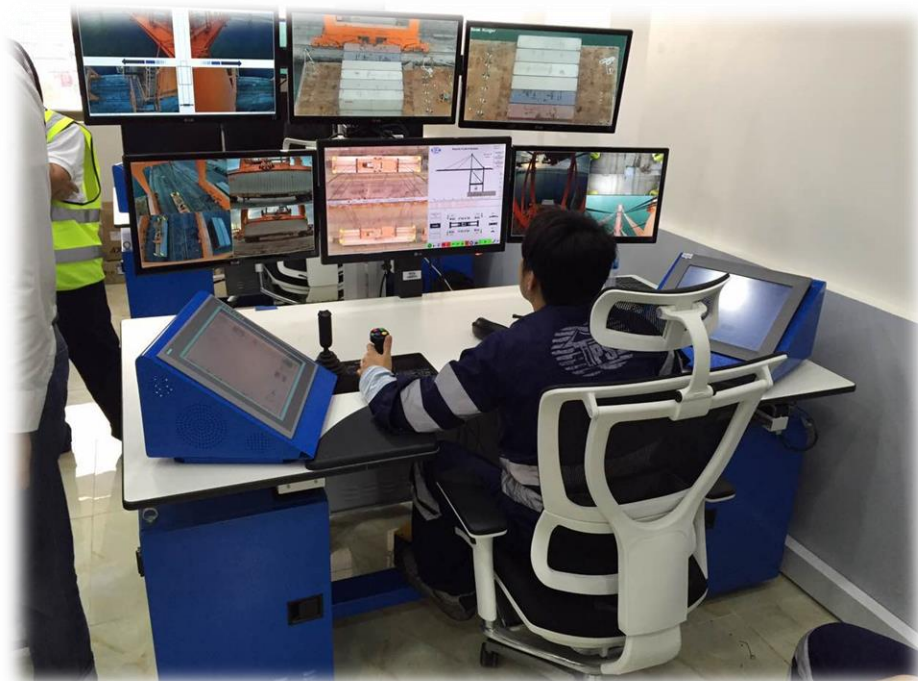
図 1 - 12 STS Remote & Automated Control System
